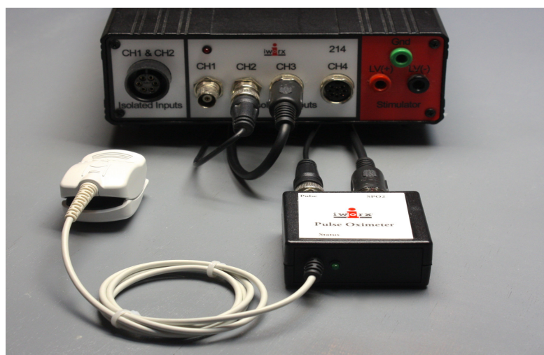
Figure HC-6-S4: A PO2100 pulse oximeter connected to an IWX/214.
