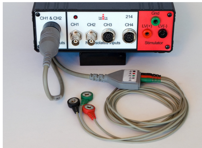
Figure HC-6-S2: A C-AAMI-504 ECG cable with 3 lead wires connected to an IWX/214.
